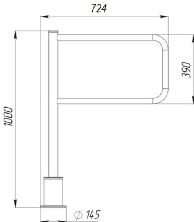
*Fig. 2 Dimensions of the gate*
